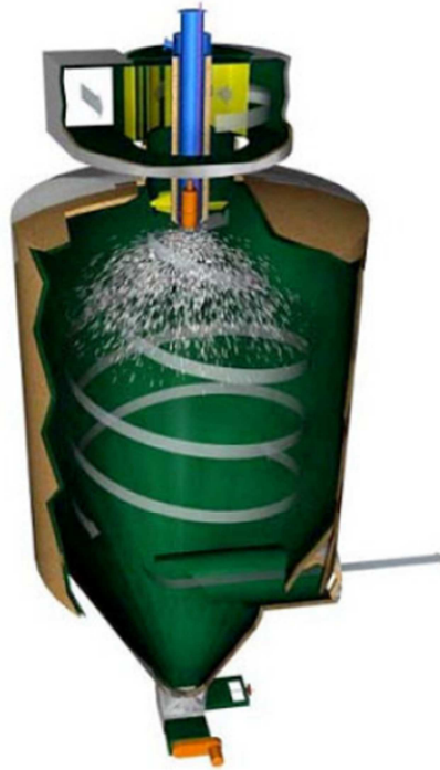
Figure 15. Reactor for semi-dry desulfurization by Keppel Seghers
